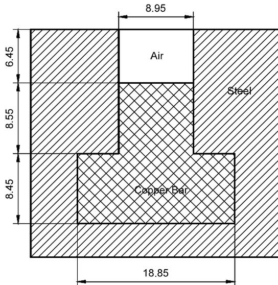
A solid copper conductor embedded in the slot of an electric machine carries a current  $I$  at a frequency  $f$ .
