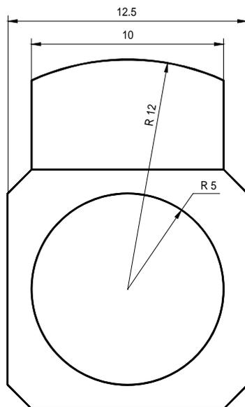
All dimensions are in millimeters and degrees Axial length of the motor is 40 mm.
