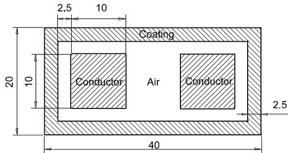
Two copper square cross-section conductors with equal but opposite currents are contained inside rectangular ferromagnetic coating. All dimensions are in millimeters.
