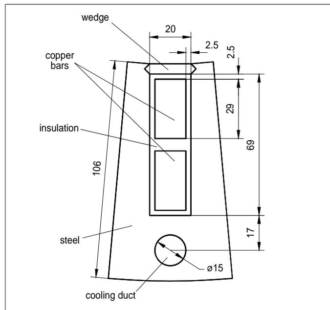
All dimensions are in millimeters. Stator outer diameter is 690 mm. Domain is a 10-degree segment of stator transverse section. Two armature bars laying in the slot release ohmic loss. Cooling is provided by convection to the axial cooling duct and both surfaces of the core.
