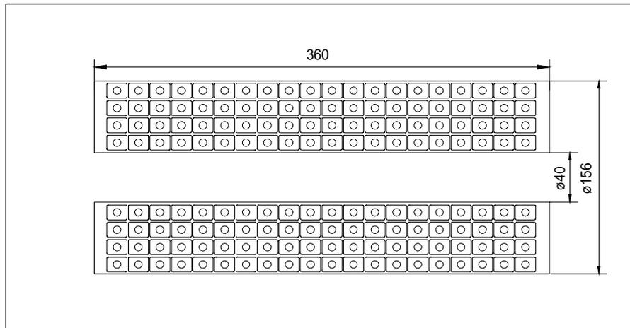
The solenoid consists of 80 superconducting coils fixed in common plastic structure. Due to mirror symmetry one half of the structure is modeled.
